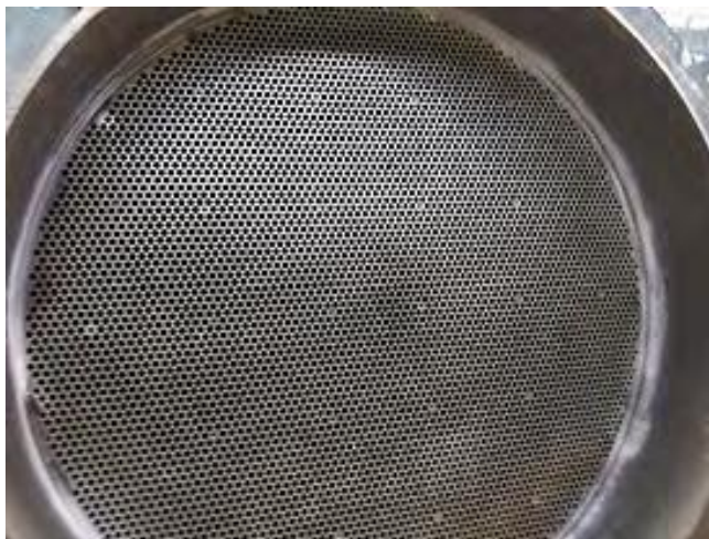
Chart 3: Critical process of fine drilling of holes of heat exchanger
