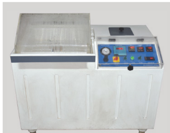
The salt spray test chamber, where components such as nuts and bolts, sheet metal and electronic PCBs are tested
