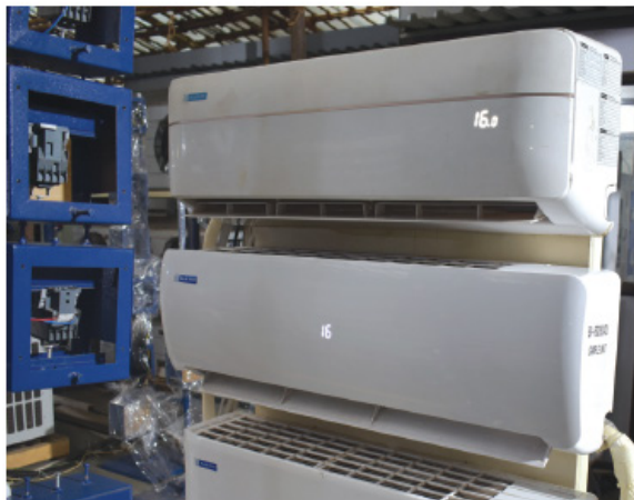
Room air conditioners undergoing endurance testing
