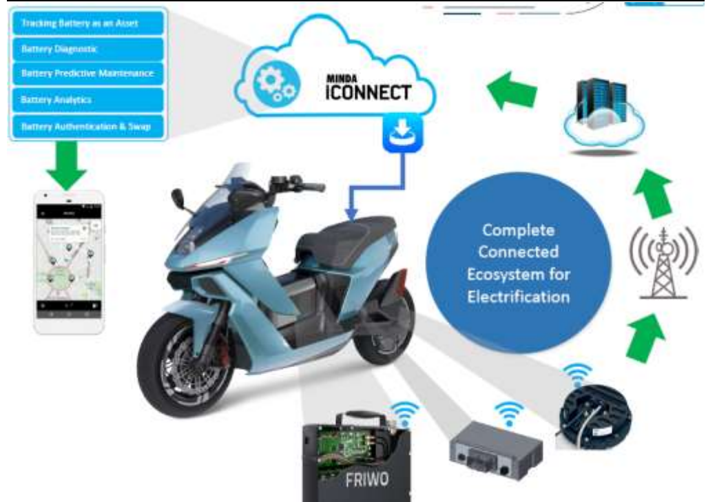
Exhibit 5: Connected solutions for EVs such as tracking battery as an asset, battery diagnostics, predictive maintenance, analytics and authentication
