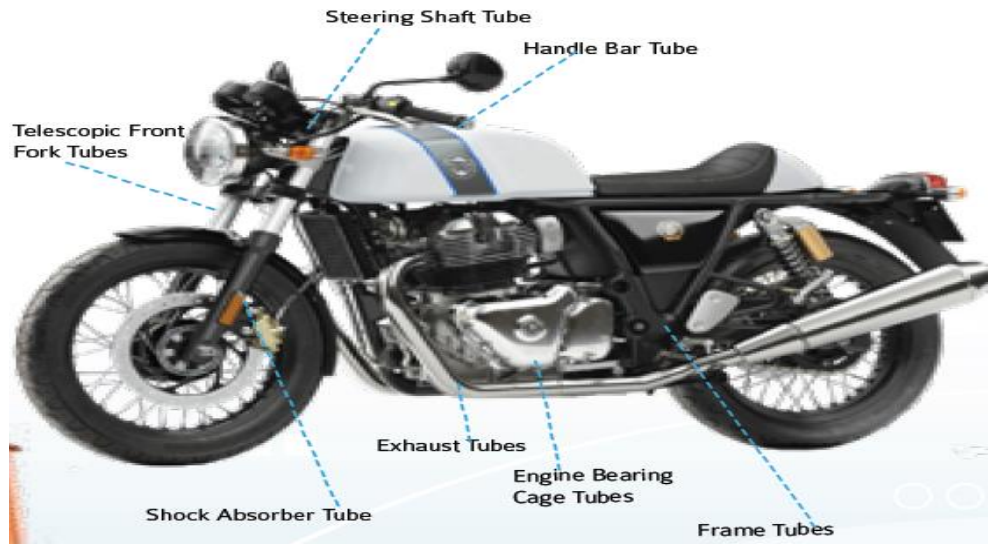
Exhibit 16: TIINDIA supplies all tubular products used in a 2W with highest market share in telescopic front fork tubes
