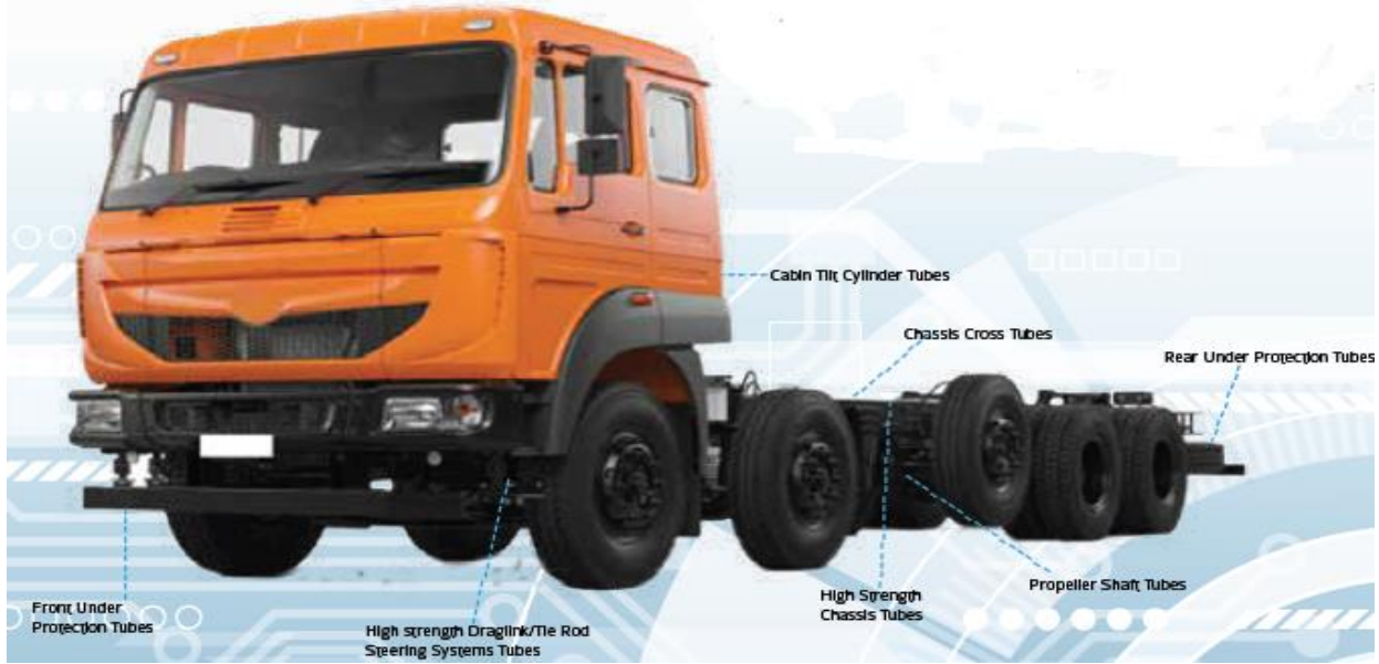
Exhibit 18: TIINDIA supplies multiple parts to all MHCV and large diameter tubes for hydraulics (used tipper trucks)
