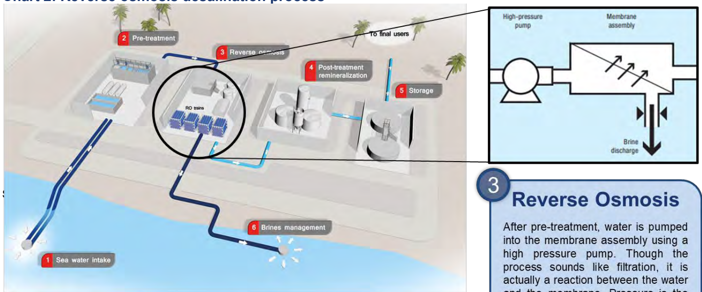
Chart 2: Reverse osmosis desalination process
