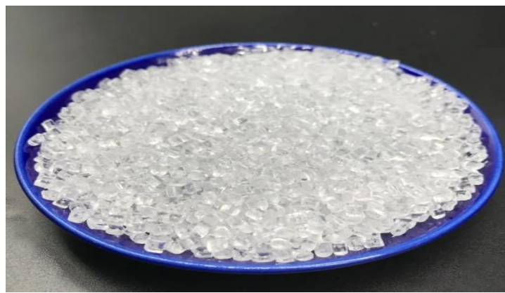
Exhibit 42: Raw materials for the body structure of a smart meter are Polycarbonate and PBT
