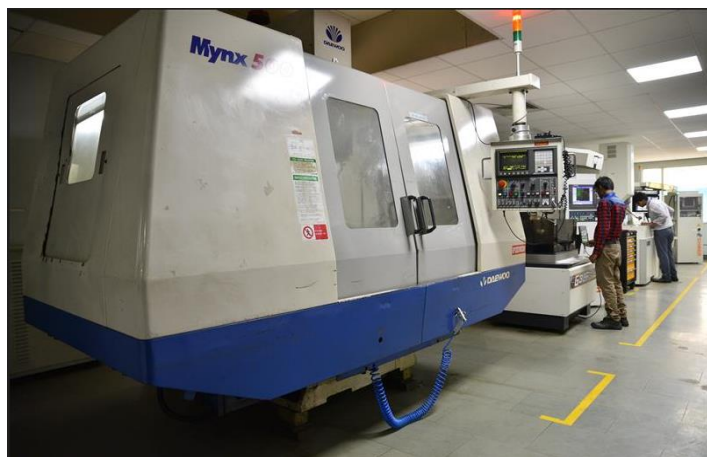
Exhibit 39: CNC machine used to mold H13 steel, basis design team working;
