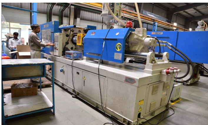
Exhibit 43: PBT Particles liquified and shaped in this machine
