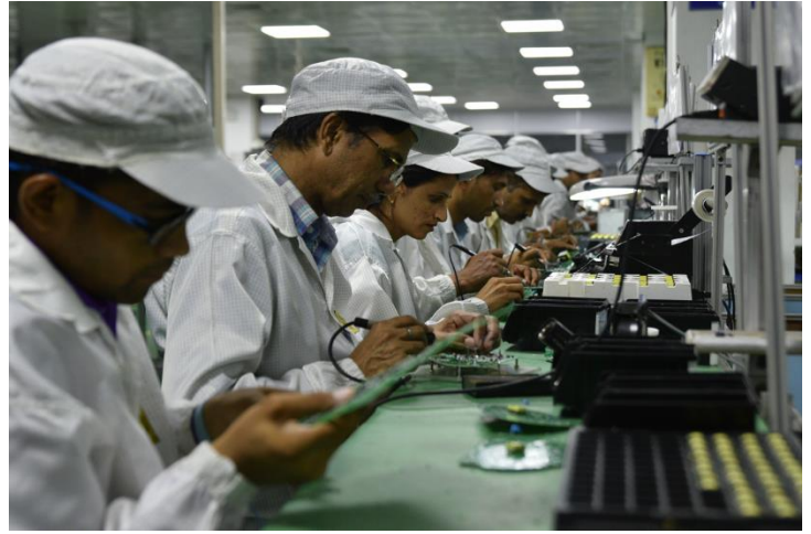
Exhibit 48: Surface mount tech (SMT) – Electrical components are mounted directly onto the surface of the PCB by workers
