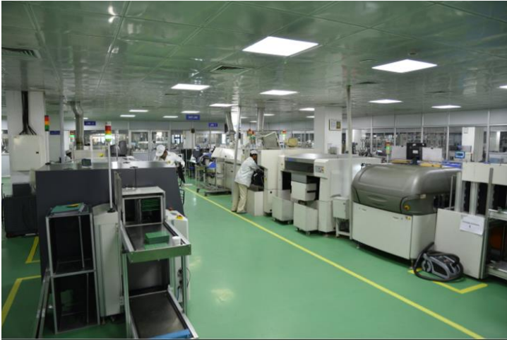
Exhibit 47: Circuit mounting of PCB through machines brought in by GPIL
