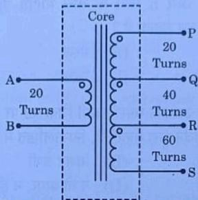
Input voltage of 20 V is applied between A and B. Between which two terminals will the output be 120 V?
