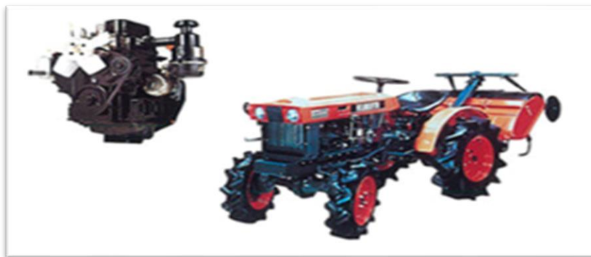
Fig 17 – Ultra-compact 4-wheel drive tractor Bulltra B6000 (right) and its vertical 2-cylinder diesel engine (left)
